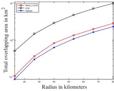
Fig. 6. Overlapping area of primary and backup path (proportional to the probability of simultaneous failure  $P_A$  as in Eq. 5) versus the radius of failure in kms.
