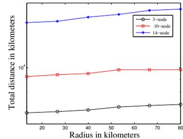
Fig. 11. Total distance versus radius of failure for 3 different intra-domain topologies at  $\alpha = 0.95$ .
