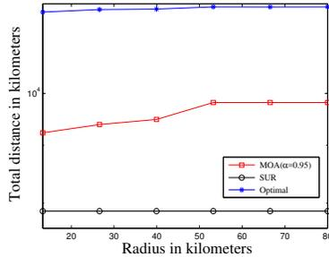
Fig. 9. Total distance of primary path and backup path versus the radius of failure in kilometers for  $\alpha = 0.95$ .
