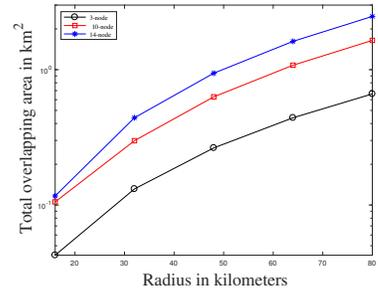
Fig. 10. Overlapping area of primary and backup path versus radius of failure in kms for 3 different intra-domain topologies at  $\alpha = 0.95$ .
