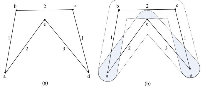
Fig. 4. (a) Primary topology aggregation which is created by selecting the minimum distance path between border nodes within a domain. (b) Secondary topology aggregation which considers the combination of minimum distance and sum of overlapping regions between border nodes within a domain.
